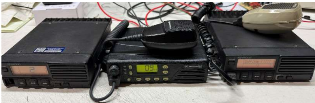
The radio lineup I've used in the past. L-R: Kenwood TK-931 (15W), Motorola GTX900 (12W), Kenwood TK-931HD (30W)
